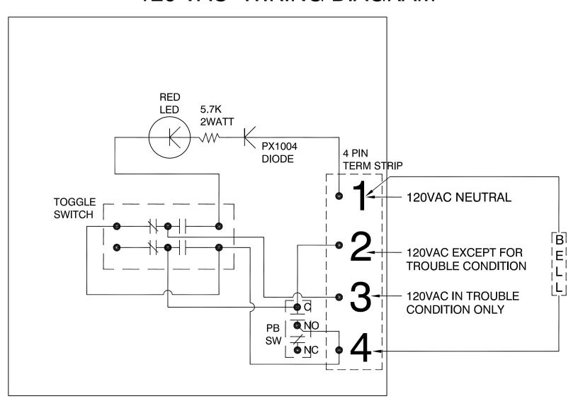
IN NORMAL POSITION BELL TEST WILL SOUND BELL. WHEN YOU GET A TROUBLE THE BELL WILL SOUND AND WHEN SILENCED THE LED WILL LIGHT. WHEN THE TROUBLE CLEARS YOU WILL GET A RING BACK UNTIL THE SWITCH IS RETURNED TO THE NORMAL POSITION.
